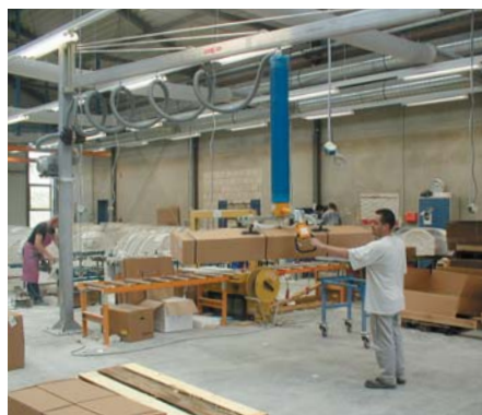
Column slewing jib SSK 125-4.000 for loads of up to 80 kgs
