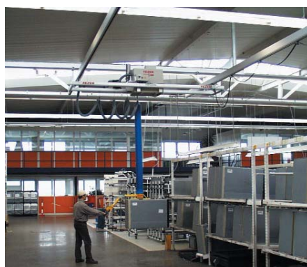
Suspension track system with double bridge and ceiling suspension. Work area: 18.000 x 5.000 mm
