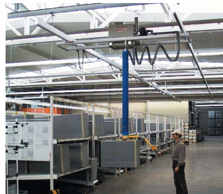
Suspension track system with double bridge and ceiling suspension. Work area: 32.000 x 5.000 mm
