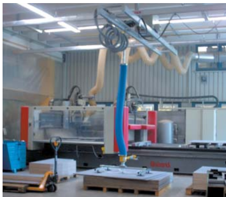
Suspension track system with ceiling suspension and double bridge. Work area: 8.000 x 5.000 mm
