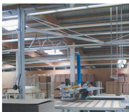
Column slewing jib SSK 125-4.000 for loads of up to 60 kgs
